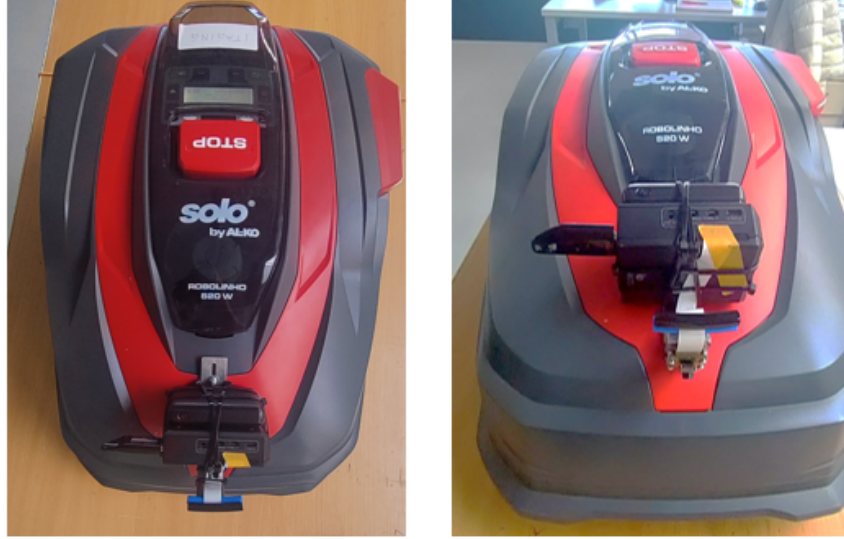
Figure 24: ROBOLINHO with Raspberry Pi 5 and Camera Module 3 Wide
