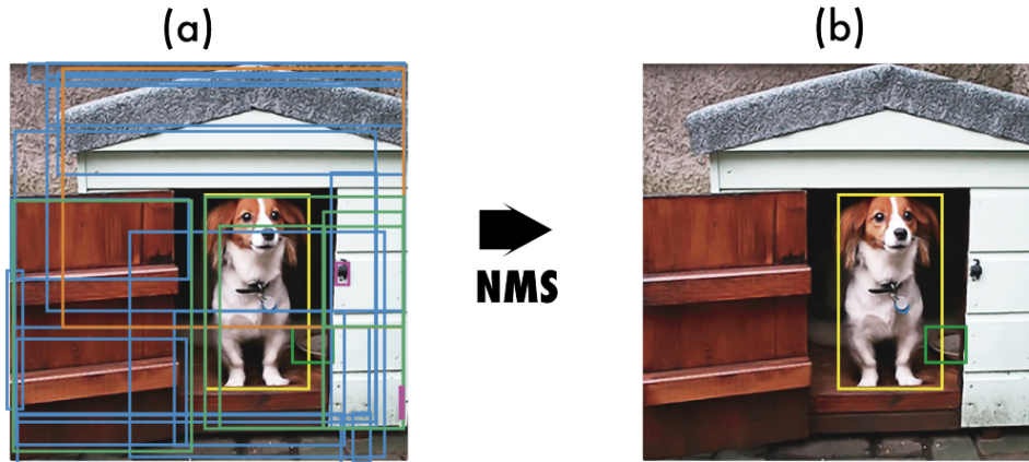
Figure 22: Non-maximum suppression (NMS). (a) Typical output of an object detection model containing multiple overlapping boxes. (b) Output after NMS. [46]
