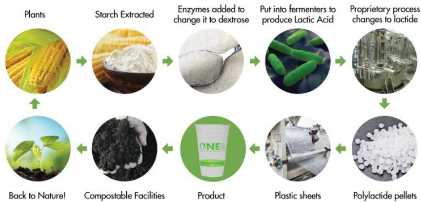
Figure 12: The Lifecycle of Poly(lactic acid) (PLA) (Din, 2020)
