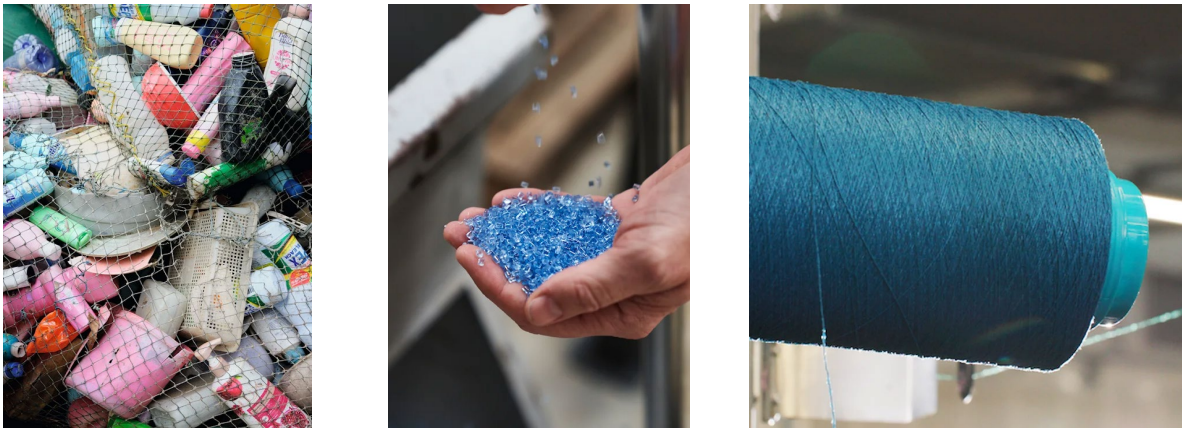
Figure 29: Kvadrat's circular process—plastic waste to yarn (Kvadrat, n.d.).
