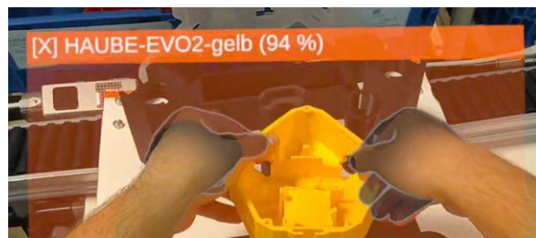
Figure 22 operator view object detection overlay – detecting a component of not the current step (self-made)
