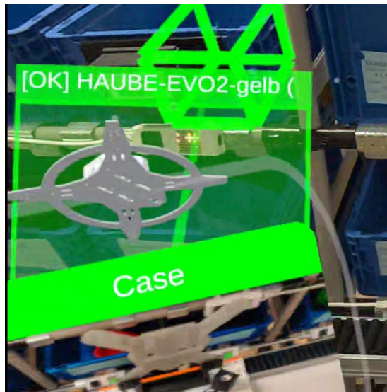
Figure 21 operator view object detection overlay – detecting the correct component of the current step (self-made)
